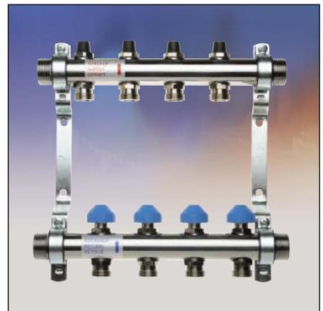
Brass or stainless steel round pipe manifolds in the sizes 1" and 1¼". Thermostat insert, regulating valve or flowmeter can be integrated. 2 – 14 outlets.
